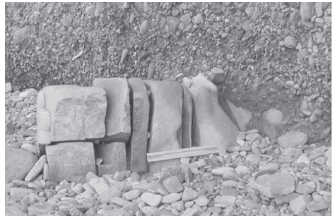
Figure 8. Close up of part of Figure 3 showing the bedrock (microgranite) joints with their raised beach matrix already deeply eroded out by wave action. The resulting joint blocks are in process of dislodgment by the sea. The scale is 25 cm long.
