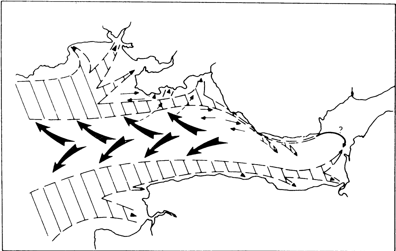
Figure 2. Conjectural near-bed sediment drift pattern, based upon the results of Woodhead drifter recovery patterns and confirmed, in places, by the movement of heavy mineral grains (from Collins and Ferentinos 1984).
